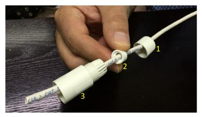
Slide the components of the seal tight kit over your network wire in the order shown in the image.
