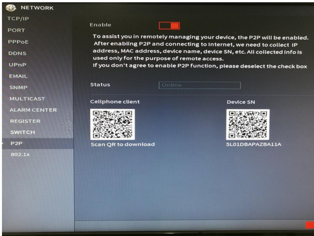
If you can't connect, something is wrong with the IP address of the machine or the network. Go to Setting then selection Network and finally click on TCP/IP and verify that you're on the right range with the right gateway. You can also activate DHCP.
